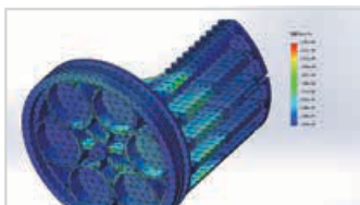
Stress of pistons analysis
