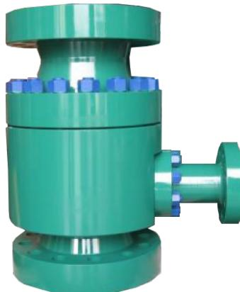
Modern industrial equipment process request centrifugal pump are basically work under condition of variable flow. An automatic recirculation valve (ARC valve) is a multifunctional valve whose primary purpose is to ensure that a pre-determined minimum flow is assured through a centrifugal pump at all times.
